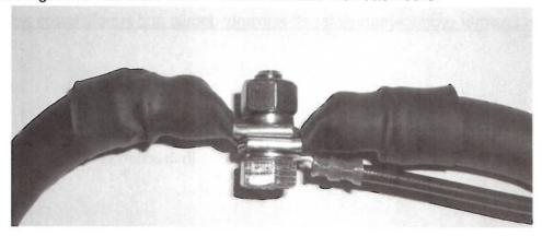
Tighten nut until the spring washer is firmly compressed.
