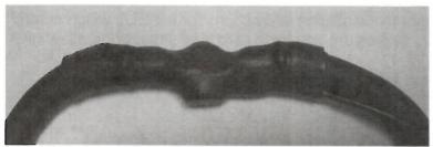
Note this join is insulated and dustproof, it is not watertight and appropriate precautions must be taken if to be fitted in a damp environment.
